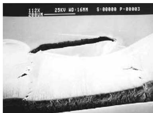
Fig. 11 Hydrogen-induced cracking. Blister crack
